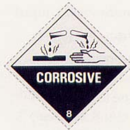
Class 8 Corrosive Materials
